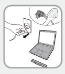
Disconnect all cables connected to the computer before cleaning it. If your notebook is an external & removable battery type, remove the external battery.
